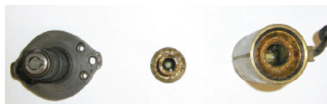
Before: Solenoid after 90 days use with previous fluid
